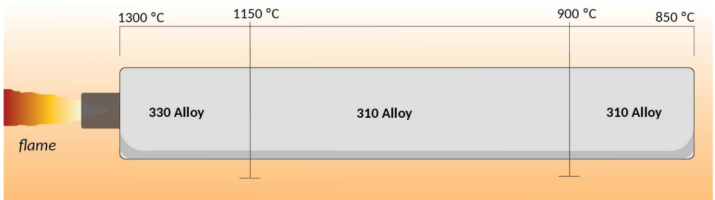
Figure 5. The above illustration depicts the recommended alloys for the burner pipe based on their high temperature properties and availability.
