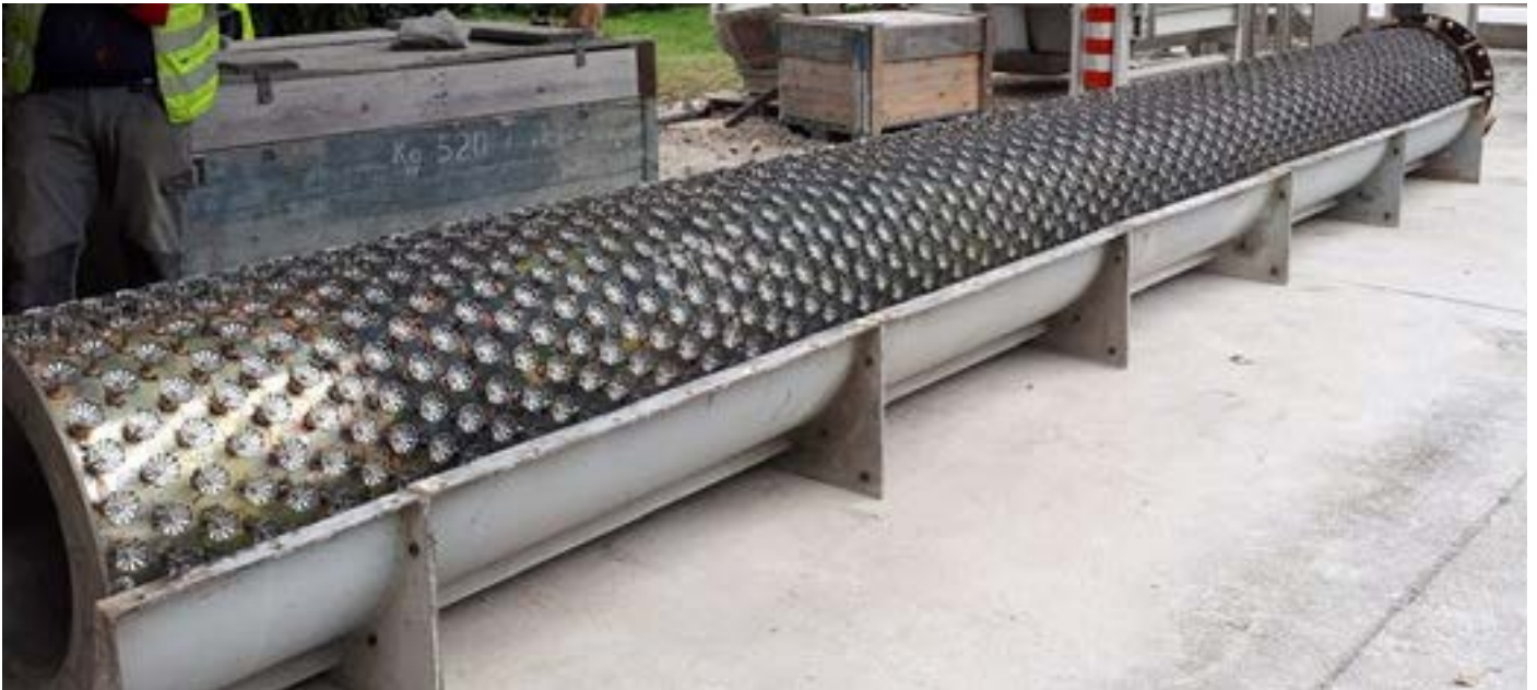
Figure 10. A fully welded pipe with SpeedCells® ready for refractory casting.
