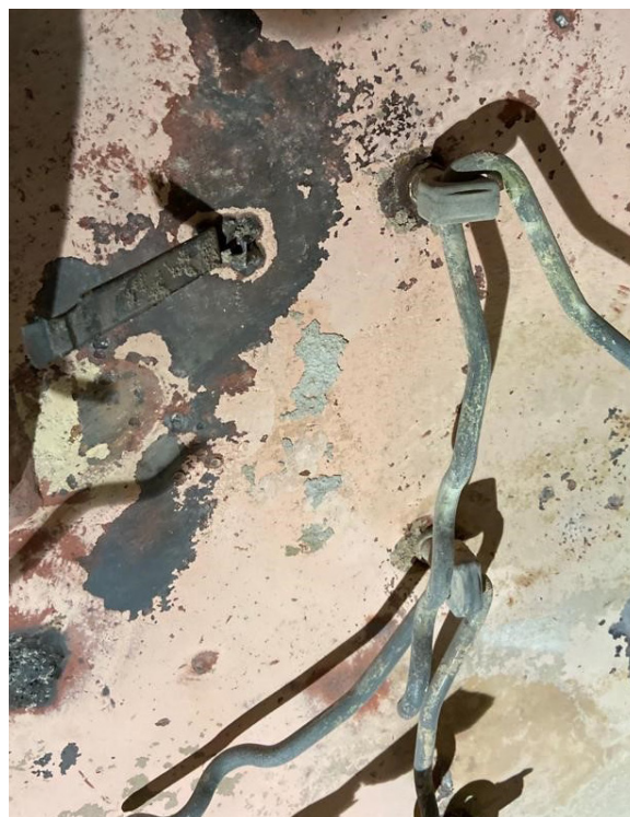
Figure 5. A bright solution annealed anchor after a few turnarounds.
